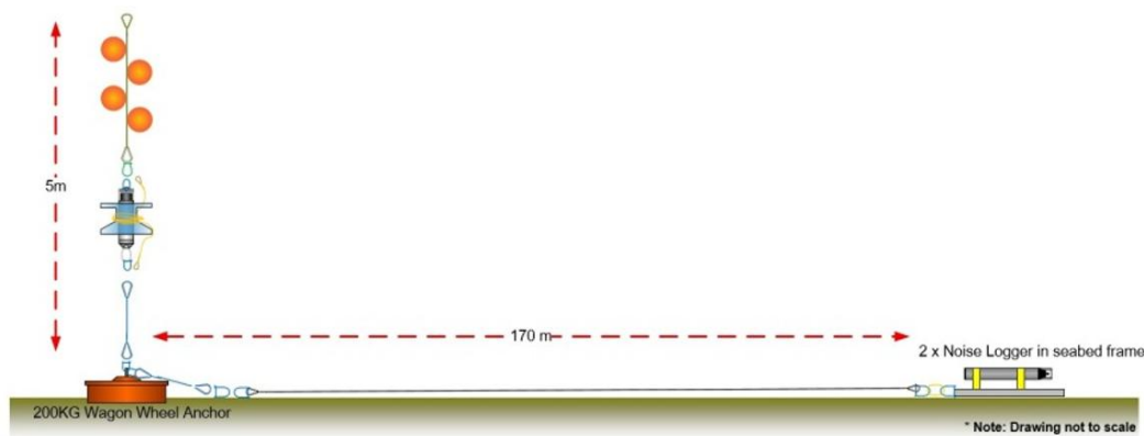
Figure 1-Design of the High Sea Wind acoustic recording stations
